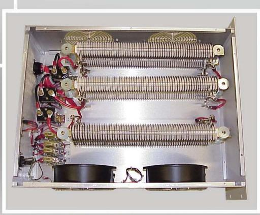
Top view of Resistive Load Unit
