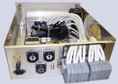
Rear View Showing Diodes on the Heat Sink
