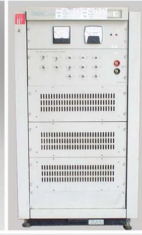
Front view of Resistive Load in Rack
