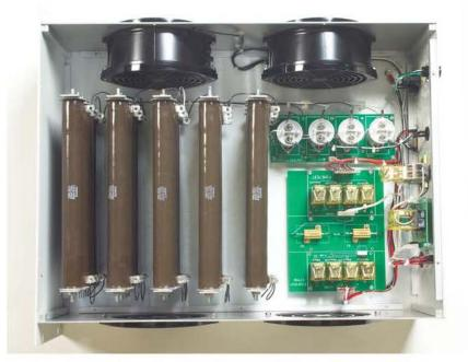
Top View showing Resistors and High Power Relays
