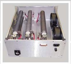
Rear view of Resistive Load Unit
