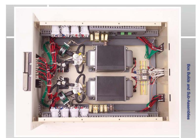
Top View showing High Current Transformers and High Power Relays
