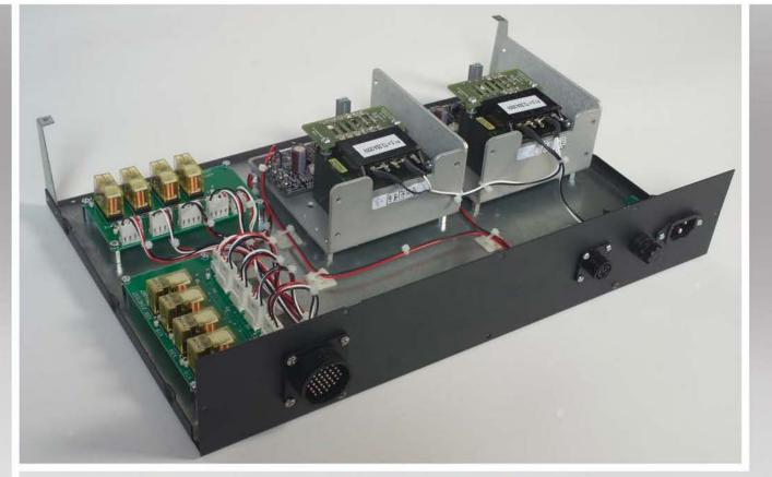
Rear Angle view of DC Mux Unit with front and cover removed
