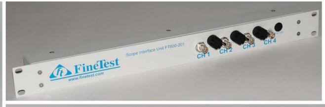
Front View of Scope Interface Unit showing scope connection BNCs and Fuses
