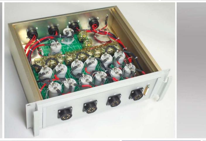
Top View with Cover Removed showing High Voltage/ High Current Power Relays
