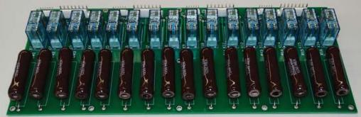
Close-Up of 1 Board with 16 Loads and the Load On/Off Relays
